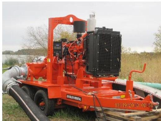
High Capacity Pump in use at State Line Lake
